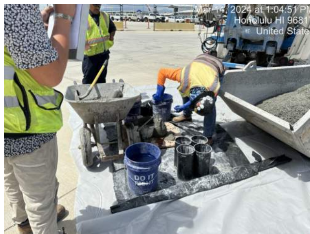
MPE performing concrete testing for the first truck of the mud mat pour of P1 of the cap beam
