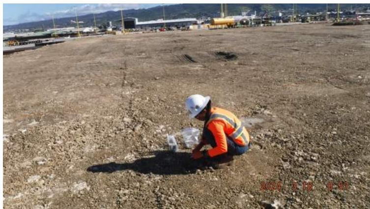
Snug Harbor: ESI environmental technician on site to collect soil samples from the 12th lift fill
