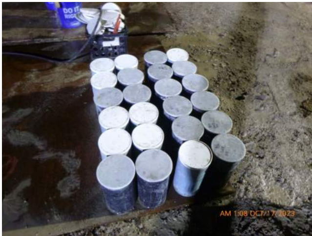
MPE taking cylinders for break testing.
