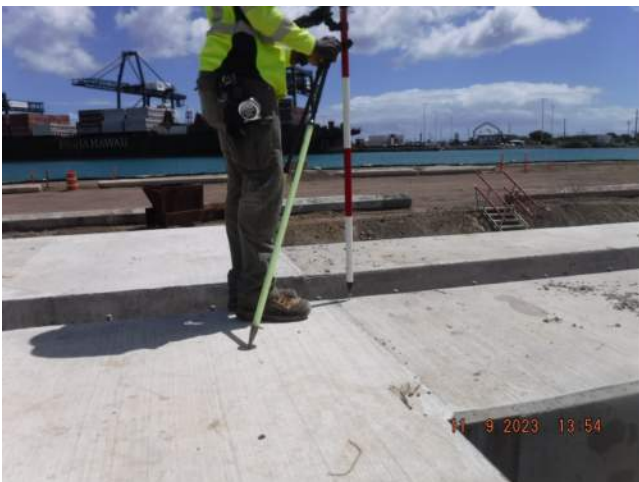
HL shooting the anchor wall to determine if it is moving
